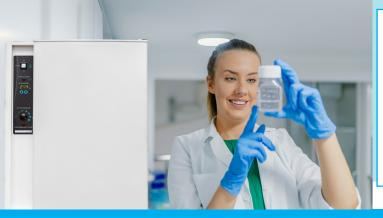
Our Refrigerated Incubators (often called B.O.D. Incubators or Low-Temperature Incubators) are used for applications such as B.O.D. Determinations, Plant and Insect Studies, Fermentation Studies, and Bacterial Culturing. SHELLAB Low-Temperature Incubator units have a temperature range of 0°C to 45°C.
