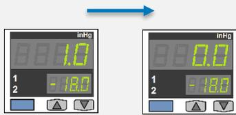
**Zero the Pressure Displays** if the BACTRON has been installed in an overpressure environment or at a high altitude. This sets the pressure gauges to local conditions. See page 47.
