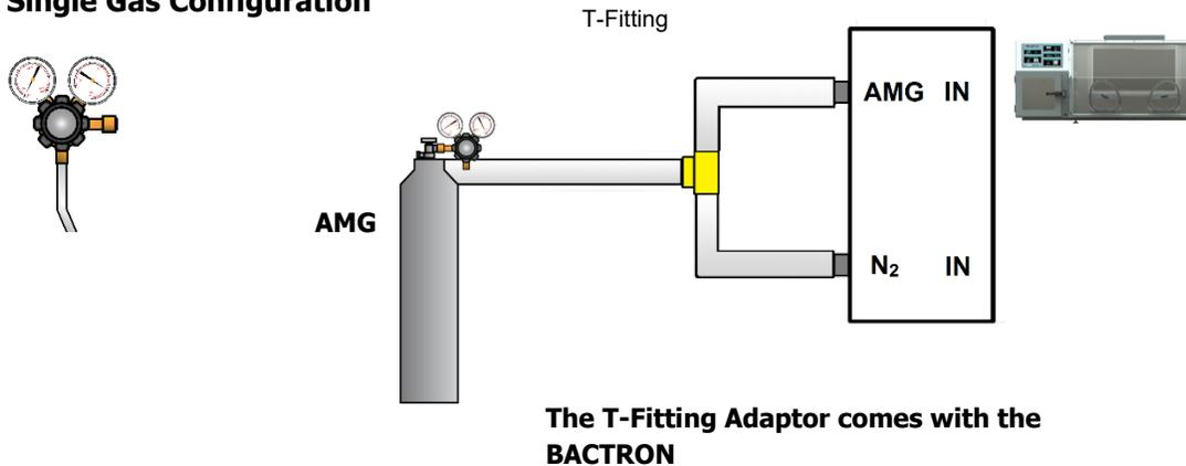
Failure to connect the T-fitting to **both** the AMG and Nitrogen In ports will interfere with the airlock auto cycle. The Nitrogen in port must always be connected to either the AMG or an N<sub>2</sub> supply.
