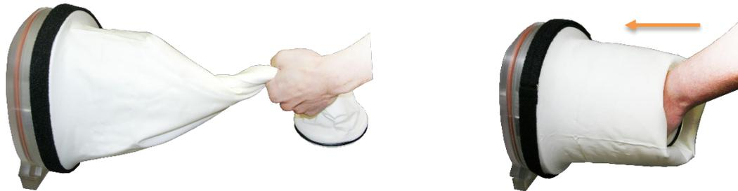
1. Grip and **slowly** push **both** sleeves simultaneously towards the doors. This will cause the sleeves to balloon.
