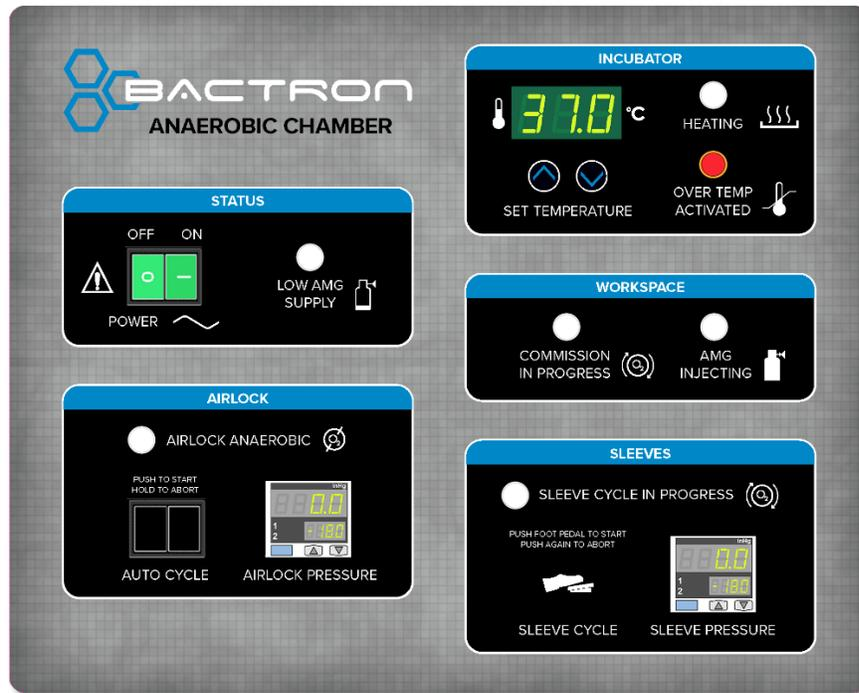
Figure 4: Main Control Panel
