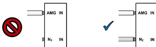
7. Verify the AMG cylinder or in-house supply regulator is set to at least 50 psi to ensure adequate pressure is delivered to the BACTRON.
