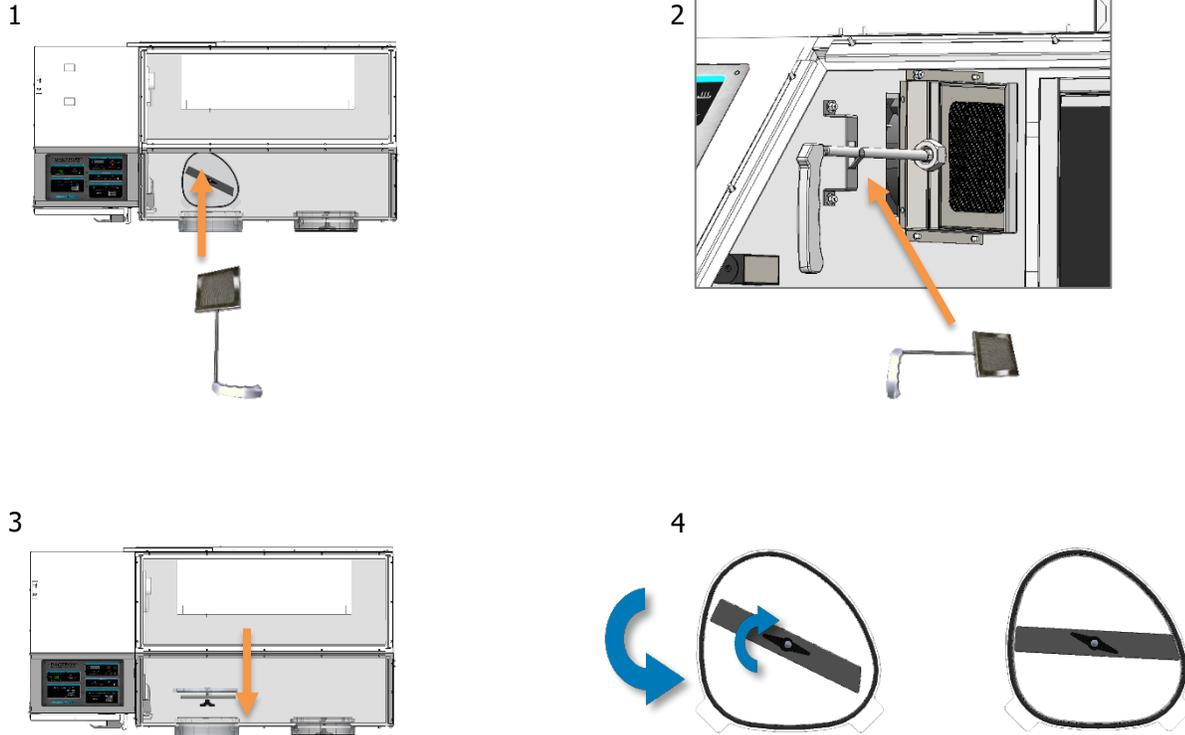
See page 29 for instructions on **properly closing and latching the arm port door**. Whenever the chamber is anaerobic, scrubbers should be introduced and removed through the airlock.
