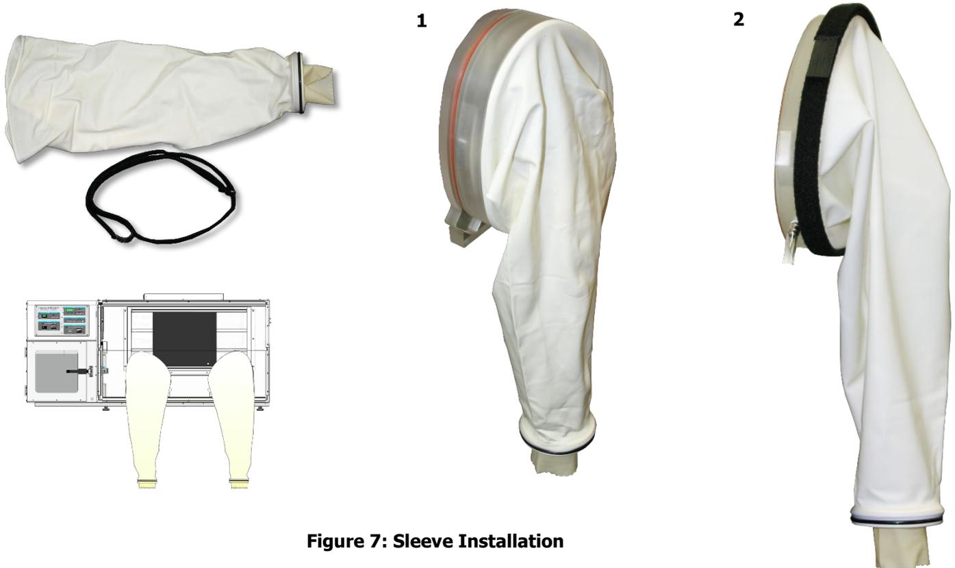
**Figure 7: Sleeve Installation**
