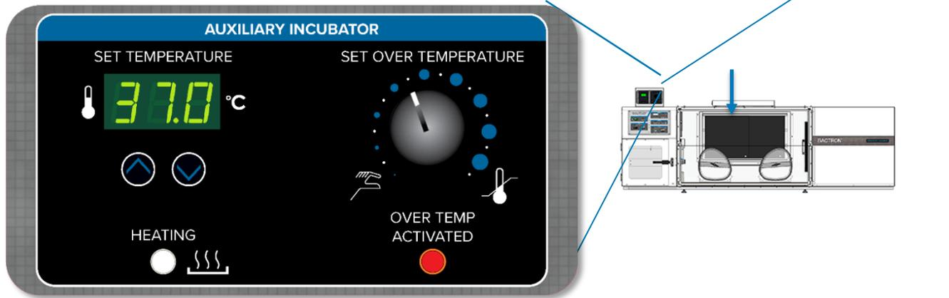
The workspace incubator control panel on the BACTRON900-2 controls the operations of the workspace chamber incubator and Over Temperature Limit system.
