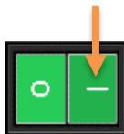
Place the Power Switch on the Main Control panel in the On ( I ) position.
