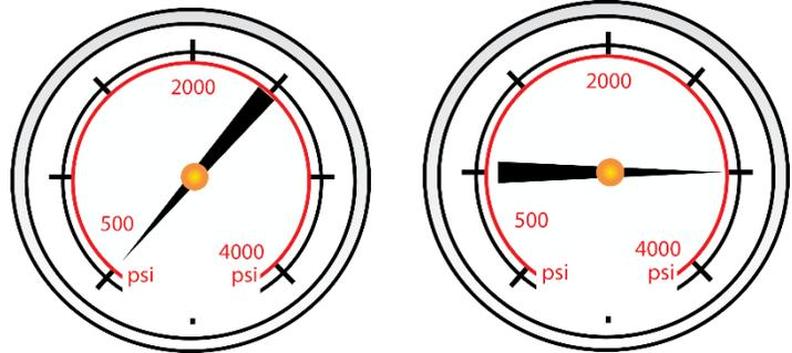
The supply gauge (right) will jump from zero ( 0 ) to showing the current gas supply pressure level.
