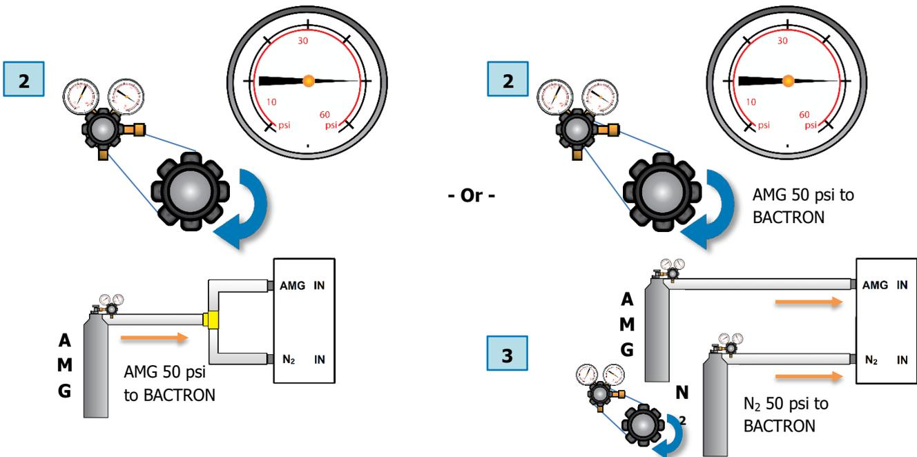
3. **Optional:** Open the Nitrogen regulator valve to supply an N<sub>2</sub> flow of 50 psi to the BACTRON N<sub>2</sub> port.
