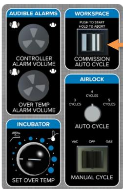
Briefly, press the Commissioning Cycle button on the side shadowbox control panel.
