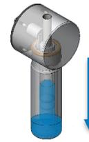
Water in manometer outer bottle forced down
