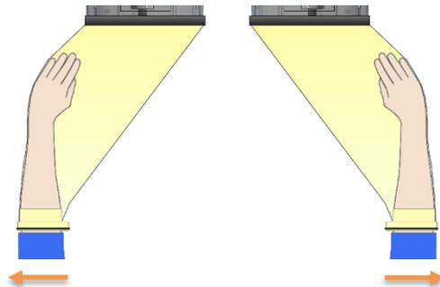
This position prevents the collapsing sleeves from pulling your hands into the arm port doors during the vacuum down cycle phases. It also keeps the sleeve material tight, helping to obtain a complete evacuation of the sleeves.
