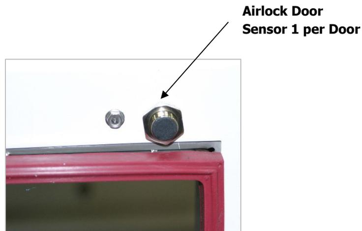
**Figure 12: Airlock Door Sensor**
