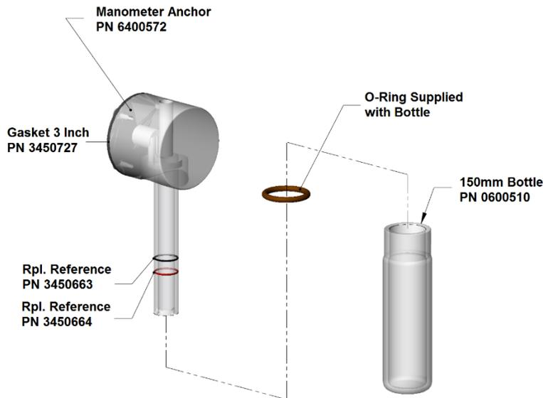
**Figure 6: Chamber Manometer**
