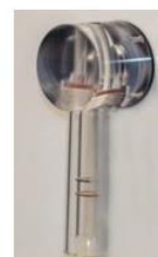
Manometer 0.5 inch (10m) water column pressure
