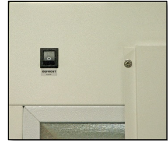
Figure 5: Defrost Cycle Switch – Top Left of Unit, Back side
